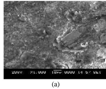
Fig.4.3: Scanning Electron Micrographs of worn surfaces of Al- 5% SiC.
