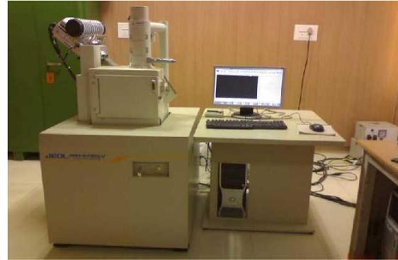
Fig.4.5: JEOL JSM-6480LV scanning electron microscope
