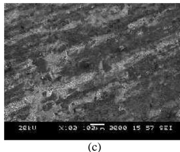
Fig.4.5: Scanning Electron Micrographs of worn surfaces of Al- 15% SiC
