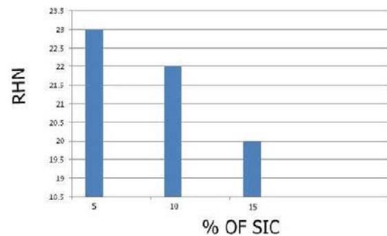
Fig. 4.1: Effect of SiC % on Rockwell hardness of the composites
