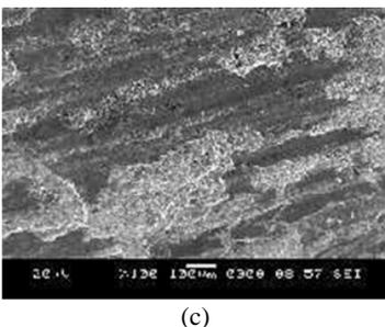
Fig.4.4: Scanning Electron Micrographs of worn surfaces of Al- 10% SiC.15%
