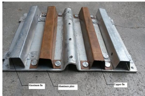
Fig 3.6 Aluminium plate with Trapezoidal fins
