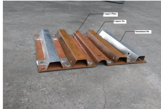
Fig 3.5 Copper plate with Trapezoidal fins
