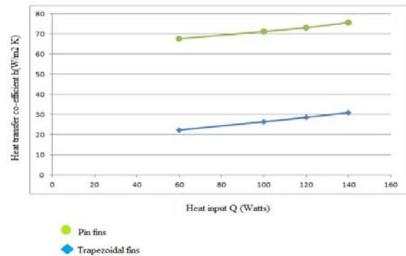
**Comparison of Heat Transfer Co-efficient for Copper plate with pin fins and Copper plate with trapezoidal fins.**
