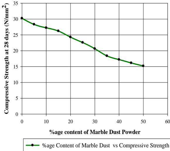
**Fig.4: Percentage Replacement of Marble Dust Powder vs Compressive Strength (N/mm<sup>2</sup>) of Concrete for M 20**
