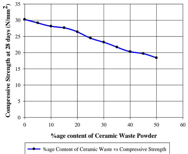
**Fig.3: Percentage Replacement of Ceramic Waste Powder vs Compressive Strength (N/mm<sup>2</sup>) of Concrete for M 20**
