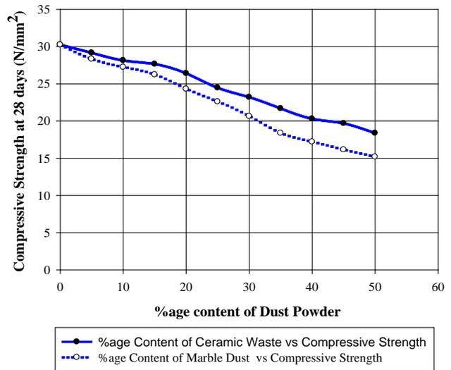
**Fig.5: (MERGE GRAPH) Percentage Replacement of both Ceramic Waste and Marble Dust Powder vs Compressive Strength (N/mm<sup>2</sup>) of Concrete for M 20**
