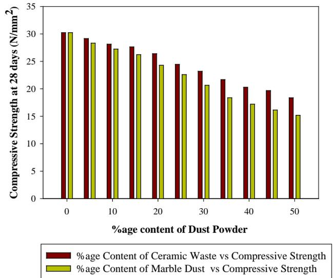
**Fig.6: (BAR GRAPH) Percentage Replacement of both Ceramic Waste and Marble Dust Powder vs Compressive Strength (N/mm<sup>2</sup>) of Concrete for M 20**
