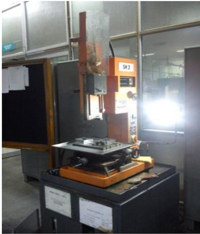
Fig 1: Micro-EDM machine
