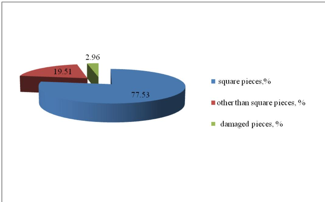
**Fig. 4 Various fractions obtained during *Sandoli* cutting**
