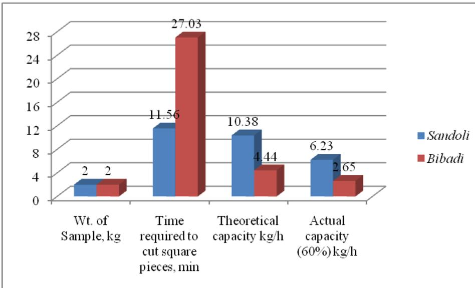
**Fig.2 Capacity of papad cutter**
