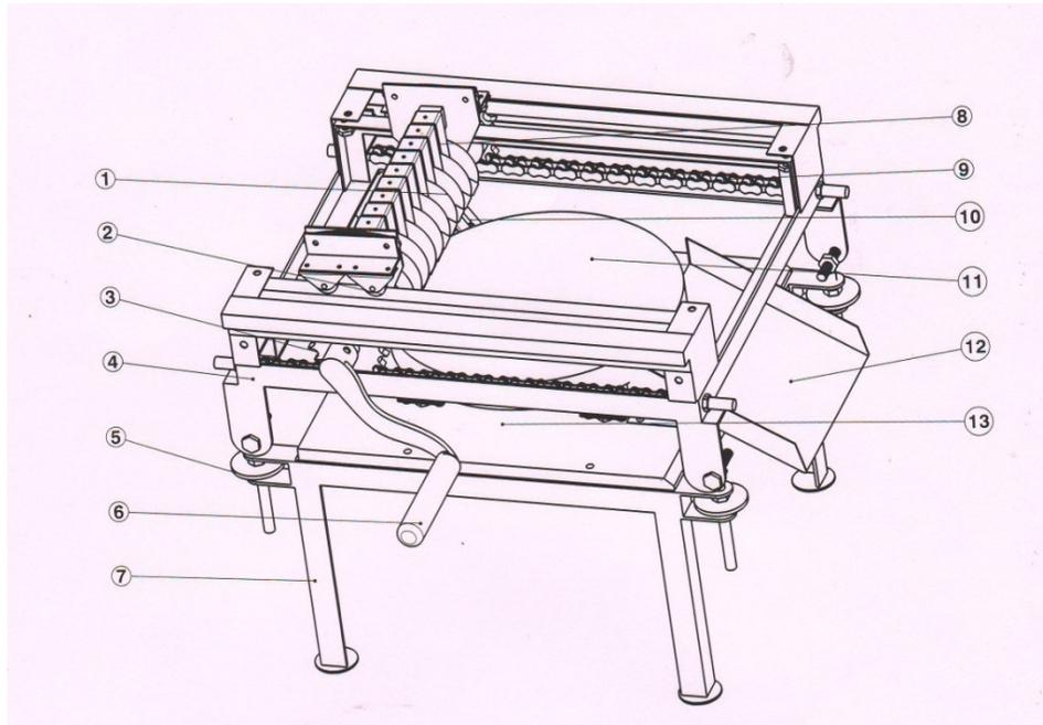
1. Circular cutting blade, 2. Fiber wheel, 3. SP Socket
