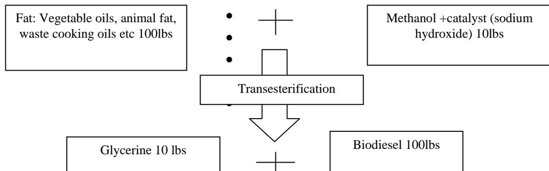
The chemical reaction that occurs through this process breaks down the oil into a layer of biodiesel which rises to the top of the reactor, and a layer of glycerine which falls to the bottom. The glycerine is drained is drained off and used for other purposes, composed or otherwise disposed off. The biodiesel is then washed, dried and filtered to remove any extra impurities and it's ready to be used as a fuel in diesel engines without any modifications to the engine.
