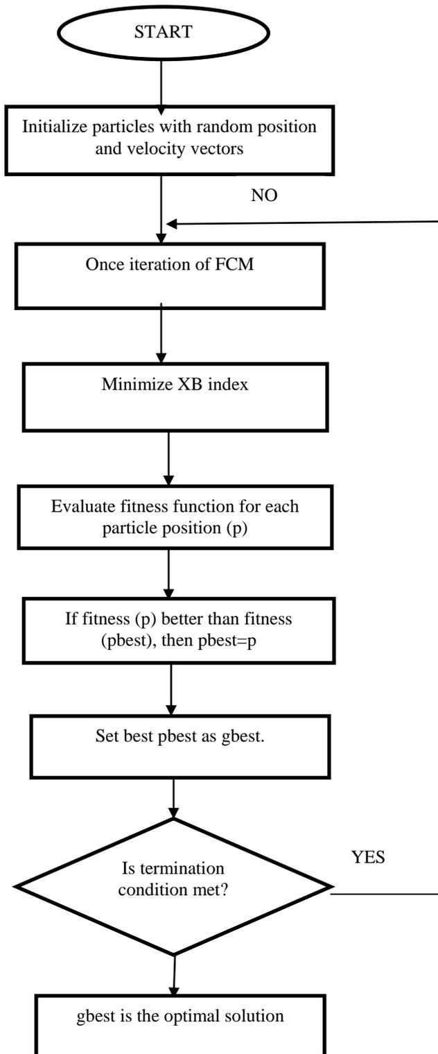
Fig. 1 Flowchart of hybrid PSO-FCM algorithm.
