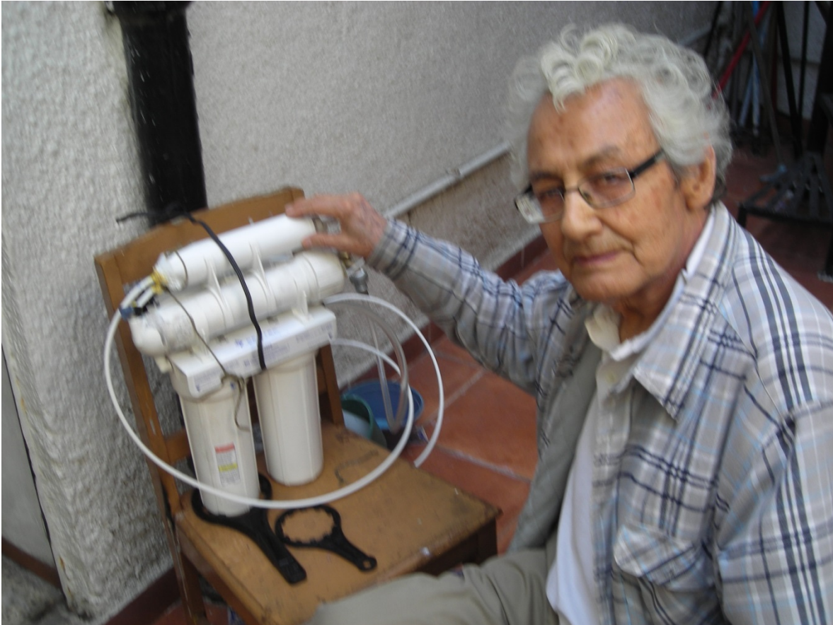
FOTHO No.-2.- EXPERIMENTAL ARRANGEMENT FOR REVERSE OSMOSIS.
