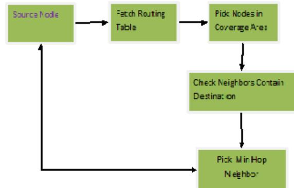
**Fig Min Hop Routing Algorithm**
