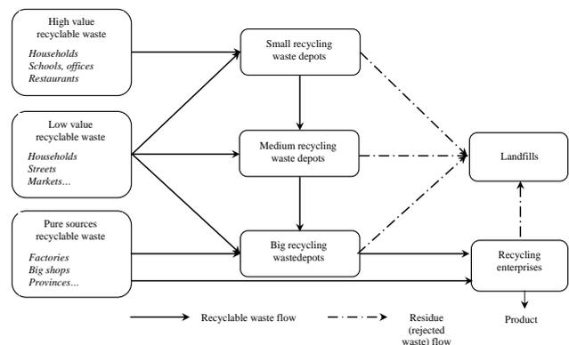
Fig. 3 Diagram of wastes reuse and recycling in Ho Chi Minh City (DONRE, 2006).
