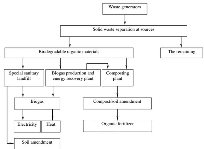
Fig. 4 A proposed solution for reuse and recycling of biodegradable organic domestic solid waste in HCMC.
