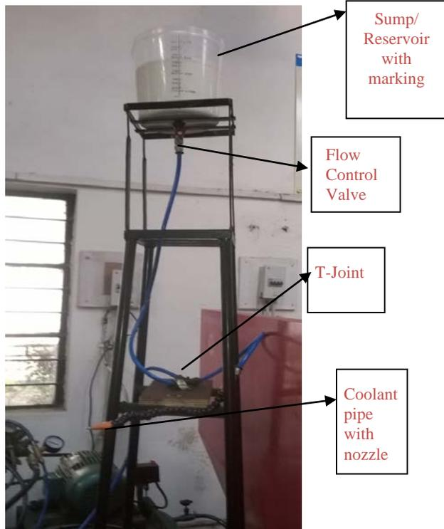
Fig.1.a: Photographic view of External MQL Set- up
