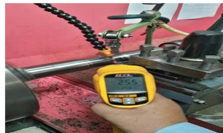
Fig.2: Measurement of temperature using K- type infrared thermometer
