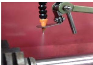
Fig. 1.c: MQL Nozzle supplying mist
