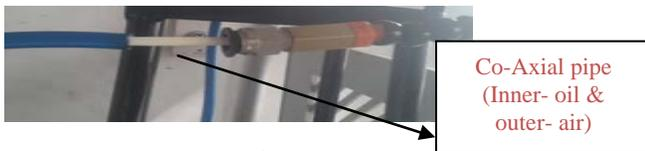
Fig.1.b: Photographic view of Co-Axial pipe
