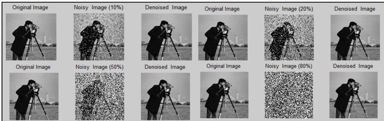
Fig 1.2 Simulation results of DBCWMF algorithm for camera-man image at 10%, 20%, 50%, 80% noise density. Noise-corrupted image; Output for parameters
