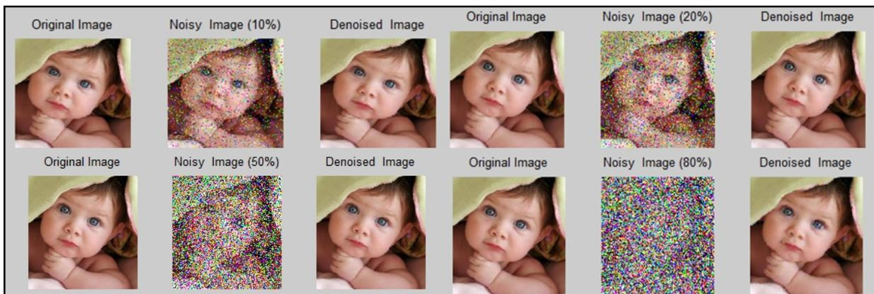
Fig1.3 Simulation results of DBCWMF algorithm for baby image at 10%, 20%, 50%, 80% noise density. Noise-corrupted image; Output for parameters
