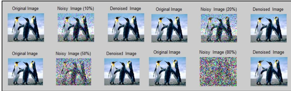
Fig 1.1 Simulation results of DBCWMF algorithm for penguin image at 10%, 20%, 50%, 80% noise density. Noise-corrupted image; Output for parameters
