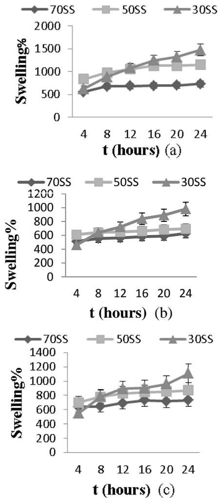
Fig 1. Effect of SNP and Temperature on Swelling Capacity of SS/PVA Hydrogel at (a) 16 °C (b) 26 °C (c) 36 °C
