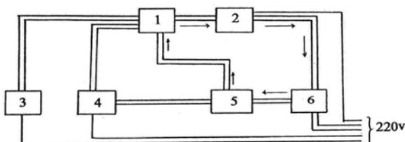
**Figure 1.** General block scheme of the polarographic device to determine O<sub>2</sub> absorption by plants: 1.electrochemical glass vessel of little volume; 2.lab pH-meter; 3.reflecting galvanometer; 4.ultrathermostat;
