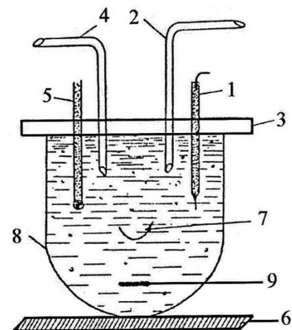
**Figure 2.** Polarographic glass vessel of a little volume: 1. Platinum electrode; 2. Plastic small tube (output); 3. Rubber stopper; 4. Plastic small tube (input); 5. Electrode for comparison; 6. Frame; 7. Circulating liquid; 8. Magnetic mixer; 9. An iron string in the small glass tube.
