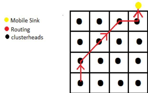
Figure 2. The selection of cluster head on the basis of shortest distance in Distance Enhancing Grid Routing scheme
