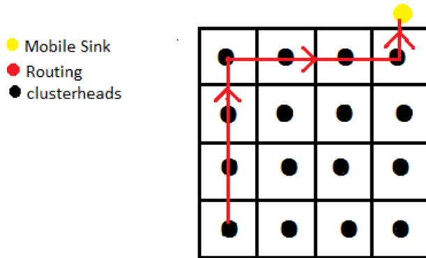
Figure 1. Straight line communication in virtual grid routing approach
