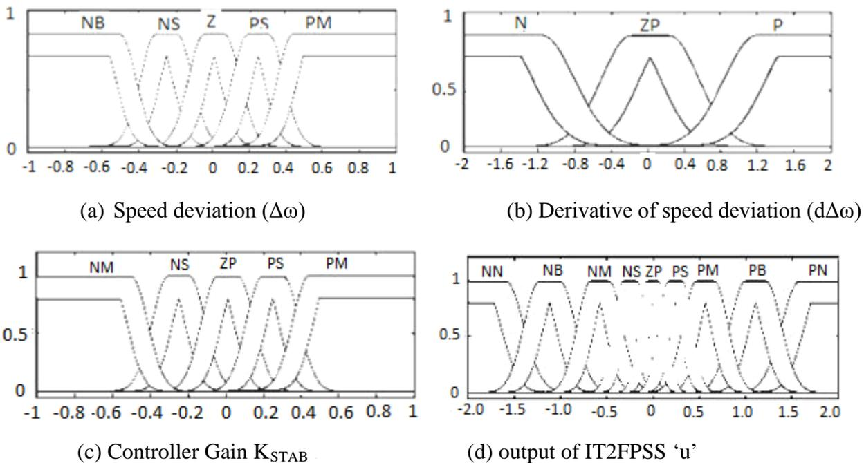
Fig. 5: Input/output membership functions
