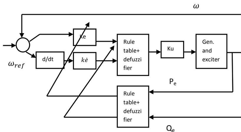
Fig. 7: Tuner for IT2FPSS using separate IT2FLS
