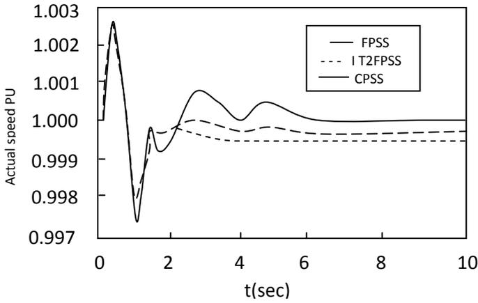
Fig. 19: Response for GEN # 1 for operating condition 2
