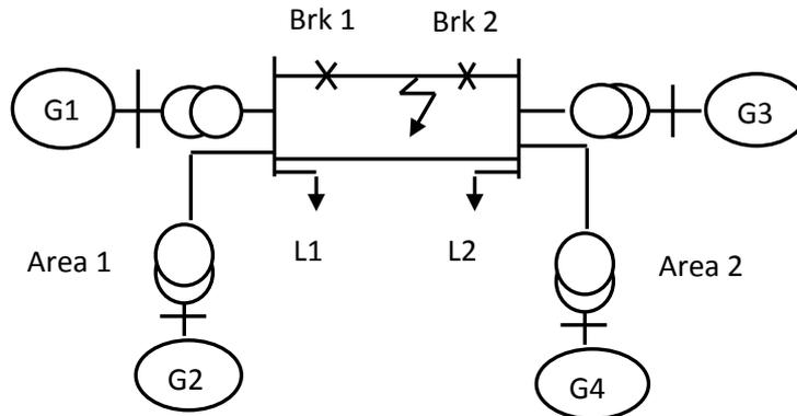
Fig. 8 Multi-machine power system for Stability study
