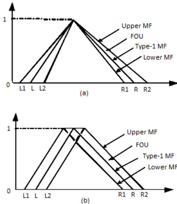
Fig.1. Interval type-2 fuzzy sets (a) Triangular MF, (b) Trapezoidal MF.
