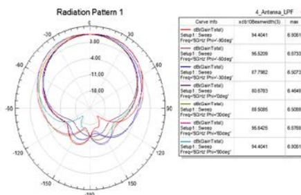
Fig 7 Combined antenna & filter response in term of Beamwidth & Gain
