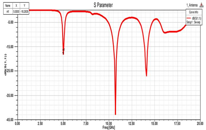
Fig 3: The S11 (return Loss) response of Pentagonal Patch antenna
