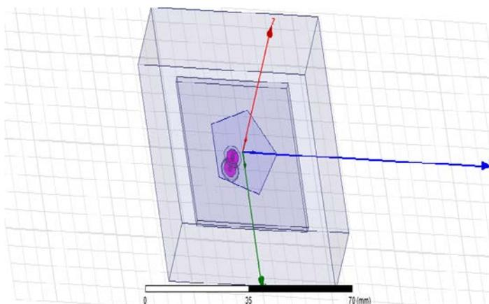
Fig 2 Pentagonal Patch Antenna
