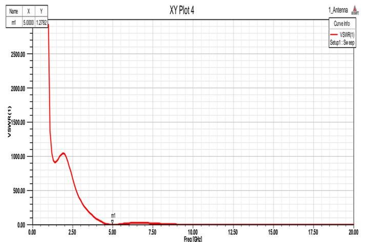
Fig4 : The VSWR response of Pentagonal Patch antenna
