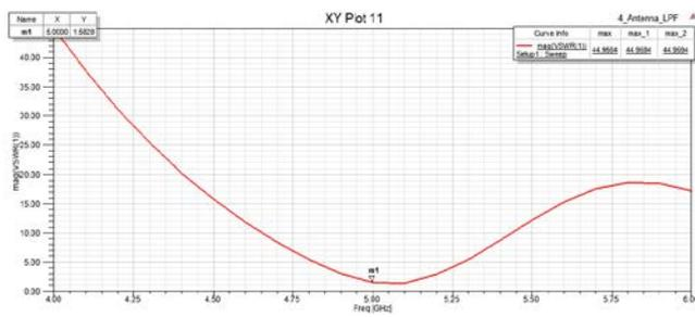
Fig 6. Combined antenna & filter in term of VSWR
