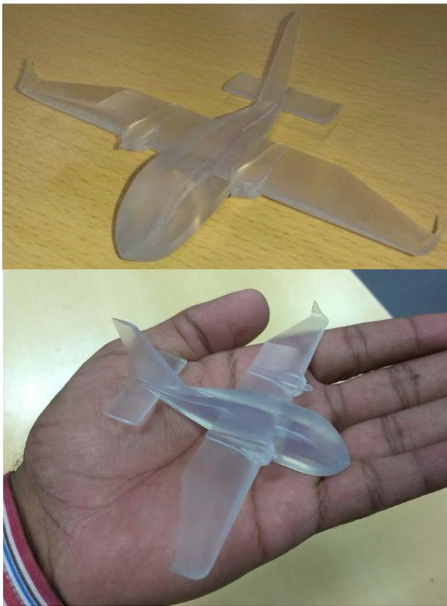
Fig. 11 The final 3D printed model of MKTS-7 aircraft
