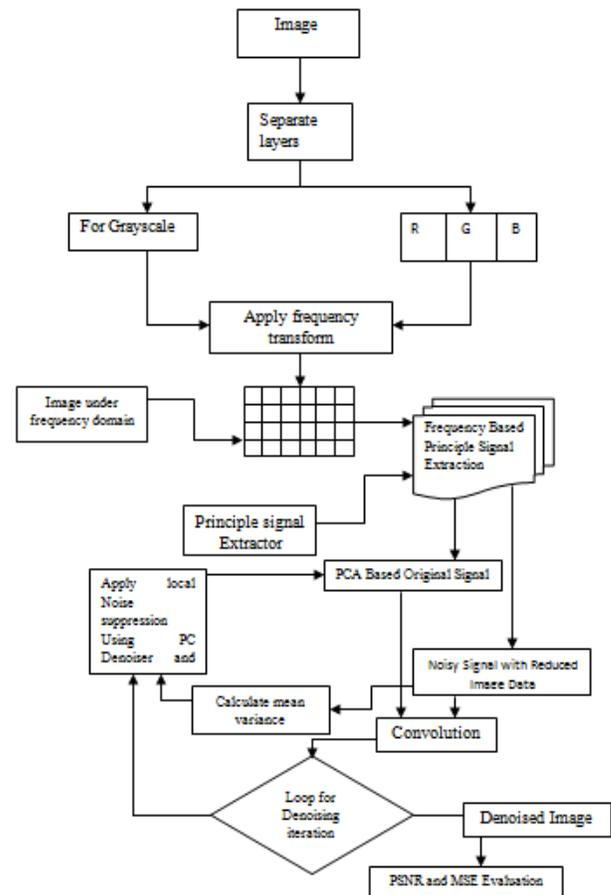
Figure 1 shows the PCA Denoiser Work Flow
