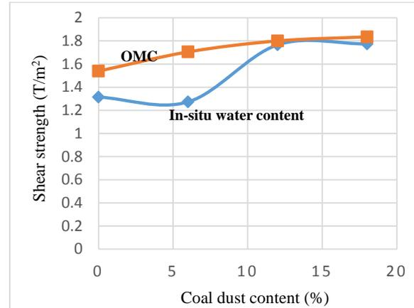
Fig. 5 Shear strength variation with coal dust content
