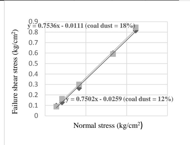
Fig. 2 Direct shear test results at in-situ water content (12% & 18% coal dust content)
