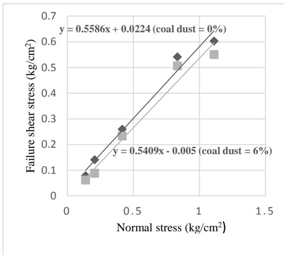
Fig. 1 Direct shear test results at in-situ water content (0% & 6% coal dust content)
