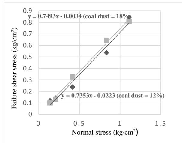
Fig. 4 Direct shear test results at OMC (12% & 18% coal dust content)
