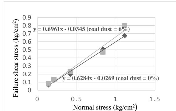
Fig. 3 Direct shear test results at OMC (0% & 6% coal dust content)
