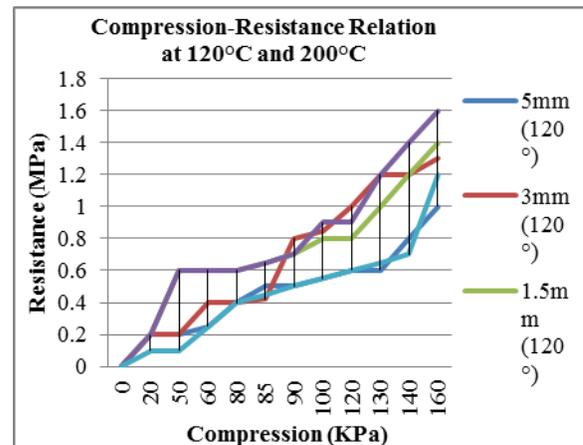
Fig. 5. Relation between compression and resistance of the material at a temperature of 120°C.
