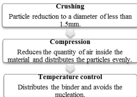
Fig. 2. Stages of thermal compression for recycling materials.
