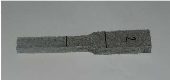
Fig. 4. Agglomerate after thermal stage
