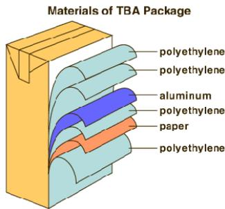
Fig. 1. Layers distribution in Tetra Brik Aseptic cartons.
