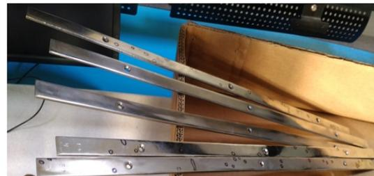
Fig 6.1: Dents on target plate of stage 1A unit-1
