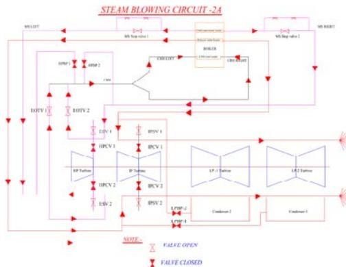
Fig 4.3: Steam blowing circuit – 2A
