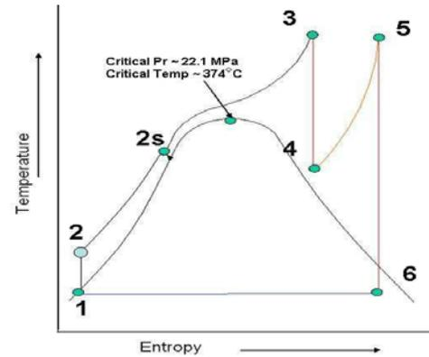
Fig 3.2: SC steam cycle temperature v/s entropy
