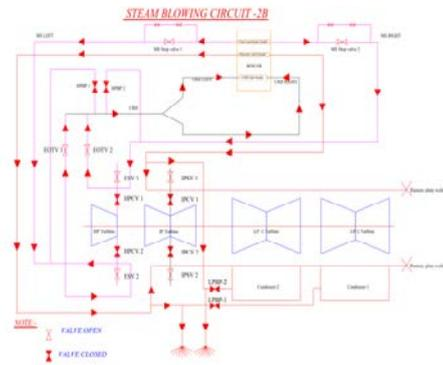
Fig 4.4: Steam blowing circuit – 2B
