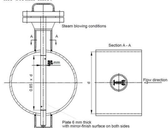
Fig 5.1: Target plate arrangement
