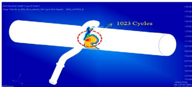
Figure 16: Staggered intermittent weld (Type B) fatigue life
