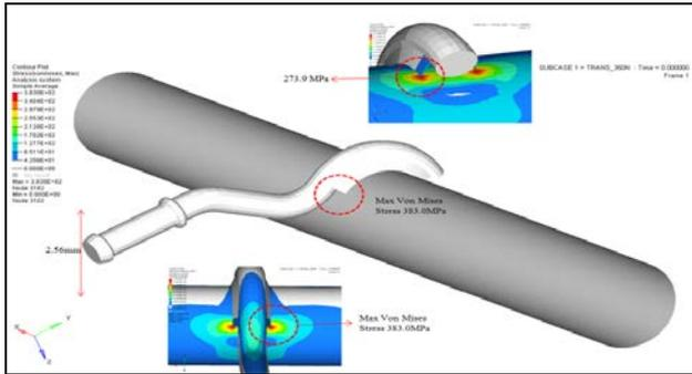
Figure 14: Intermittent double fillet weld (Type D) stress plot
