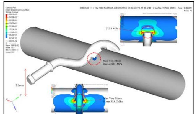
Figure 13: Two side full weld (Type C) stress plot
