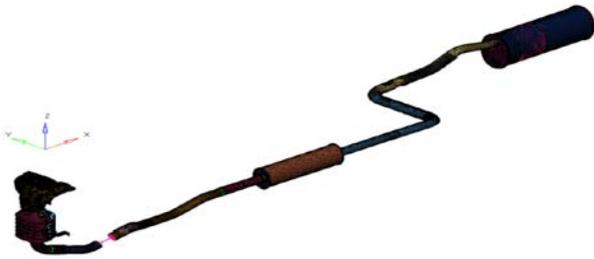
Figure 3: Represent the hanger location predation boundary condition (Inlet flange bolt holes are constraint in all degrees of freedom)
