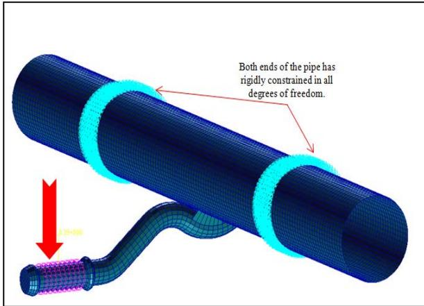
Figure 10: Loading condition of hanger rod
