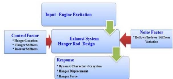
Figure 2 : P-Diagram of exhaust system design
