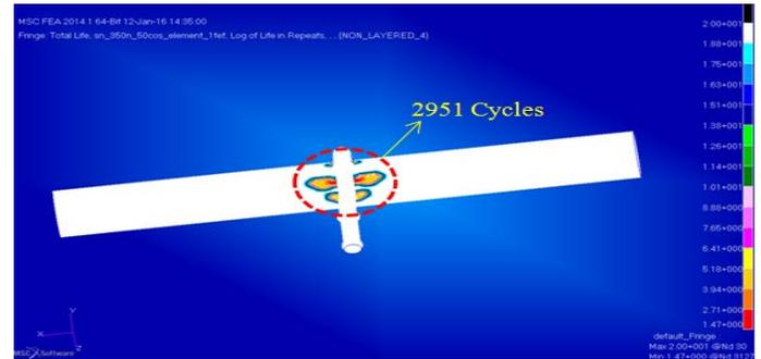
Figure 18: Intermittence double fillet weld (Type D) fatigue life
