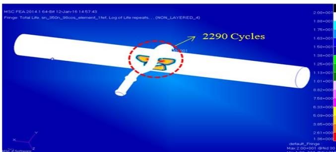
Figure 17: Two side full weld (Type C) fatigue life
