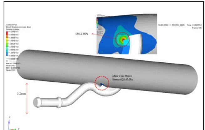
Figure 12: Staggered intermittent weld (Type B) stress plot
