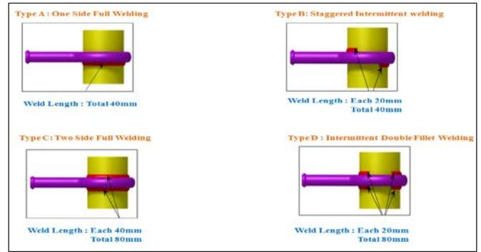
Figure 7: Different weld length for hanger rod to pipe
