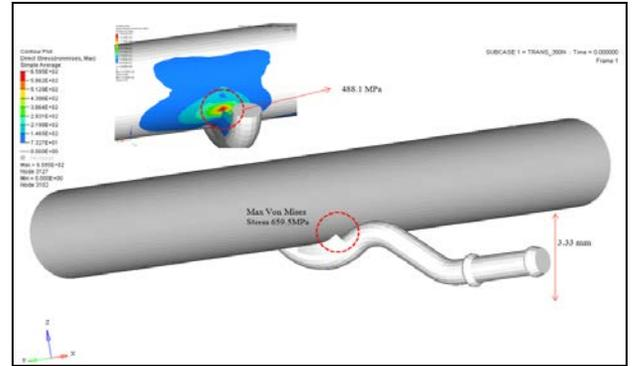
Figure 11: One side full weld (Type A) stress plot
