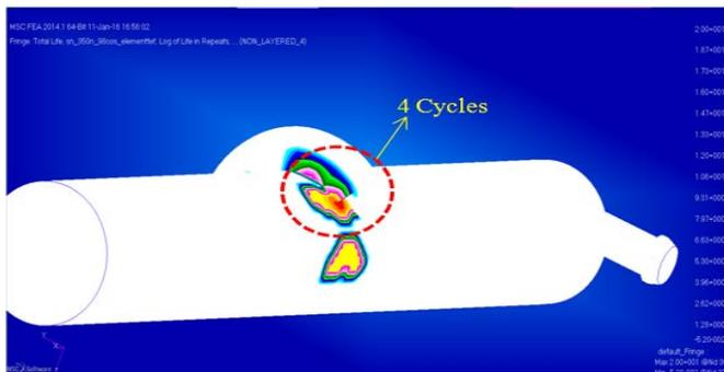
Figure 15: One side full weld (Type A) fatigue life
