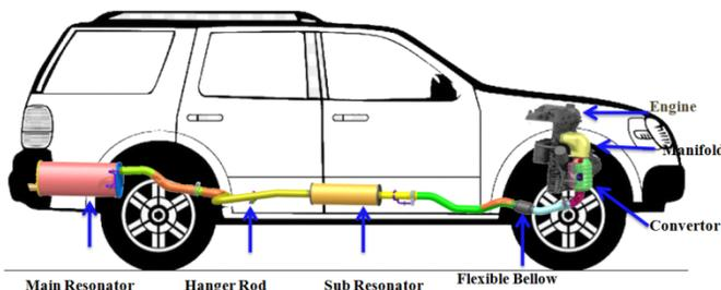
Figure 1: Represent the exhaust system in vehicle
