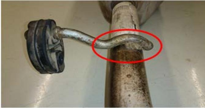
Figure 6: The pipe to hanger rod weld
