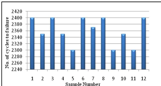
Figure 23: Two side full weld (Type C)
