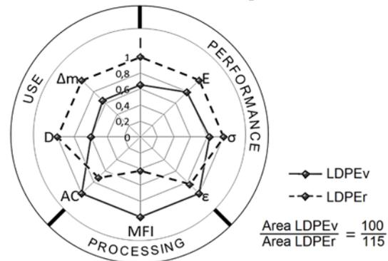
Fig. 6 Environmental "fingerprint" of the results from the virgin and recycled LDPE composites with MMT (3 wt.%).
