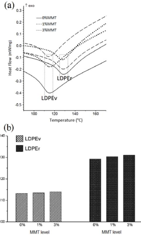
Fig. 3 (a) Principal part of the DTG curves of the samples. (b) Crystalline melting temperature ( $T_m$ ) for virgin and recycled LDPE and their composites with MMT (1 and 3 wt.%).
