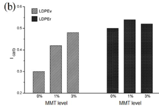
Fig. 1 (a) Crosslinking density formation and (b) carbonyl formation.
