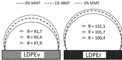
Fig. 4 CA results for the virgin and recycled LDPE and their composites with MMT (1 and 3 wt.%).
