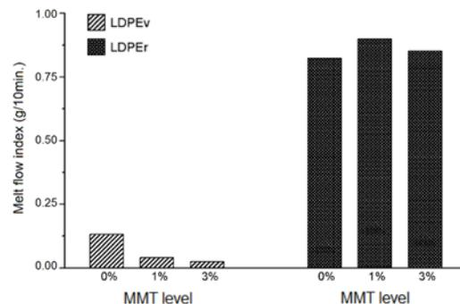
Fig. 2 MFI values for virgin and recycled LDPE and their composites with MMT (1 and 3 wt.%).
