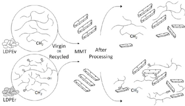
Fig.7 Proposed model for the virgin and recycled LDPE composites behavior with MMT.
