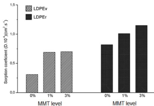
Fig. 5 Sorption results for virgin and recycled LDPE and their composites with MMT (1 and 3 wt.%).
