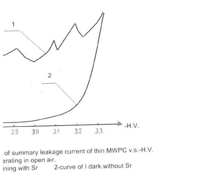
In Fig.3 shows the curve of the efficiency of registration with beta source of  $Sr^{90}$  in the gas mixture Ar+20%  $CO_2$  for confirming of the good state of the detector. We can see that plateau of efficiency reaches the value of about 250 volts indicating a well-chosen design of the detector to compare with previously samples. The curve 2 shows the value of the dark current when detector operates without a source of radiation.
