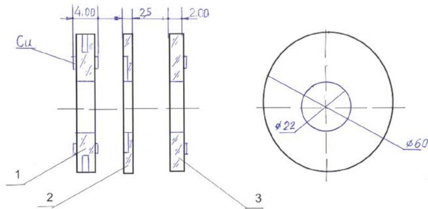
Fig.1. A schematic view of thin MWPC composition from 3 main elements.
