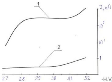
d leakage current of thin MWPC in gas mixture Ar+20% CO2
