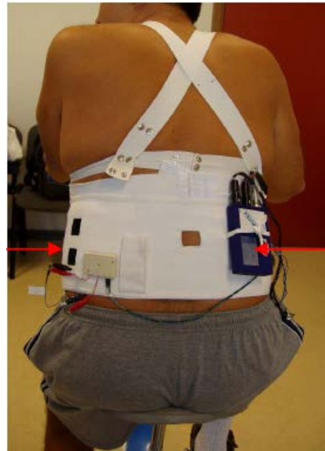
Fig.7 Experimental set-up, sweat rates sensor is positioned on the left, the pH textile patch on the right behind the control unit.
