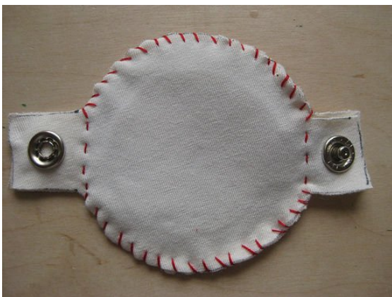
Fig. 9 Conductive fabric pressure sensor. Conductive fabric and anti-static plastic are sew together.
