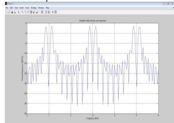
Fig 4. cognitive radio primary user spectrum
