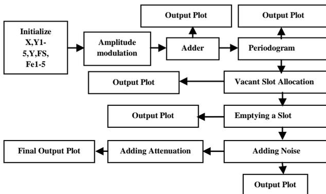
Fig 3. Methodology/Block diagram of simulation set up.
