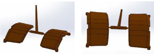
Fig. 3 Tail lamp lens with proper feeding system
