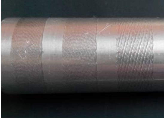
Fig. 13 The aluminium sample, processed by vibromechanical finishing with feed rates of 0.008, 0.012 and 0.016 mm/rev (from left to right), at a rotation speed of 71 rev/min
