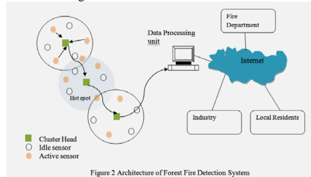
Figure 2 Architecture of Forest Fire Detection System
