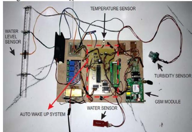
Fig 4. Top view of proposed project
