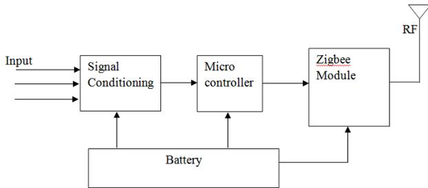
Figure 1. Wireless Sensor Networks using Zigbee
