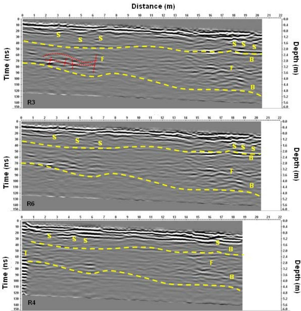
Figure 5. The processed radar sections related to the profiles named R3, R6 and R4
