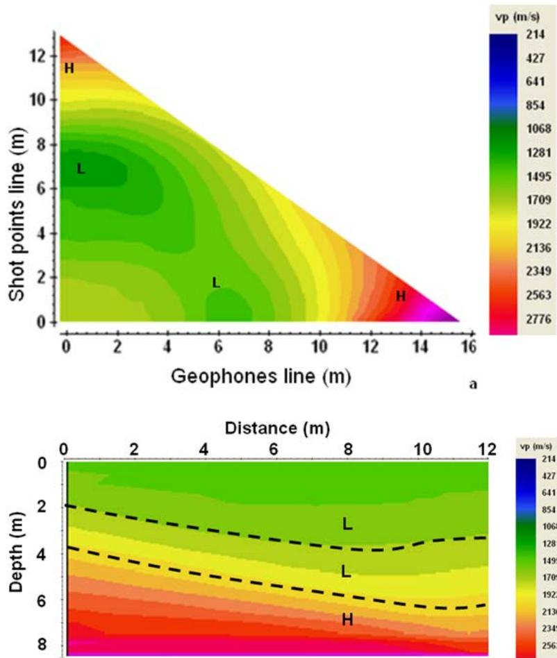
Figure 6.  $v_p$  distribution model: a) in the surveyed area; b) at the shot point line
