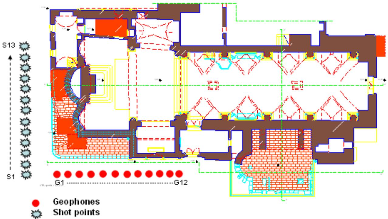
Figure 4. Seismic refraction tomography acquisition geometry
