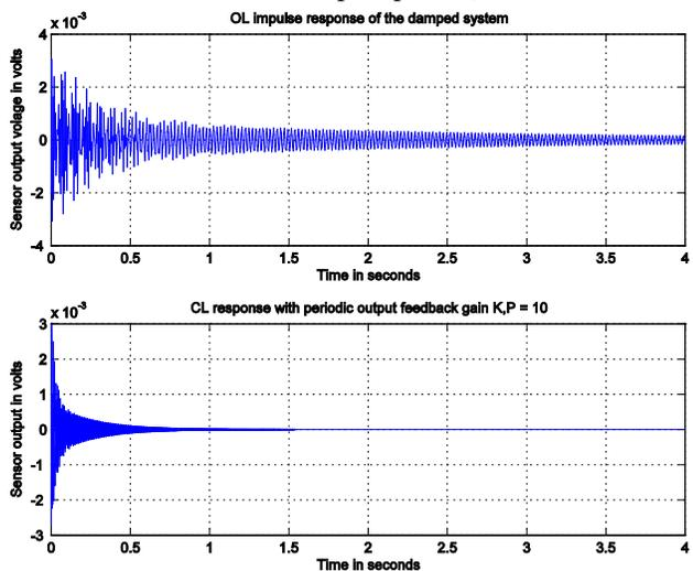
Fig. 3 : Sensor outputs at FE positions 5 (Open loop & closed loop responses)
