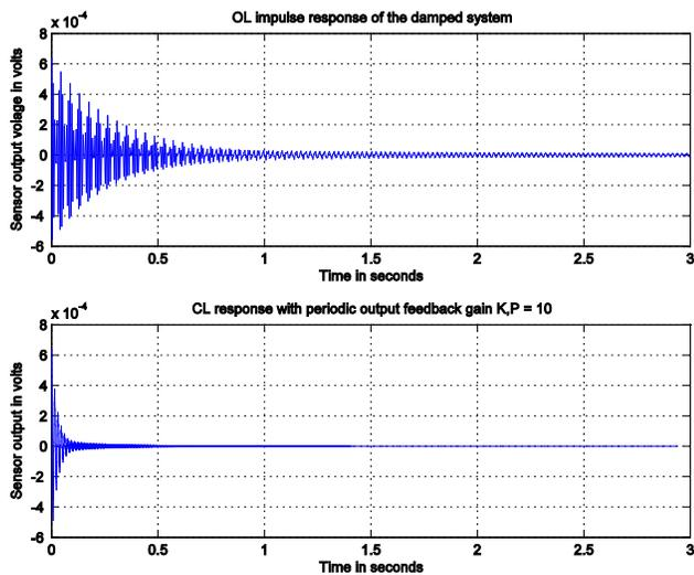
Fig. 2 : Sensor outputs at FE position 10 (Open loop & closed loop responses)
