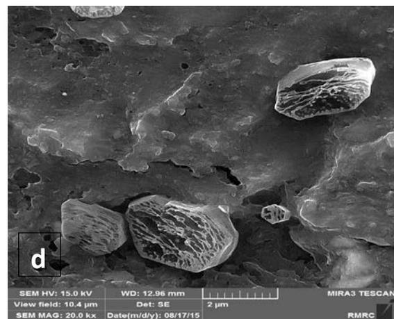
**Figure 4: SEM images for 2024 Al alloy with B<sub>4</sub>C powder (a) 500 x magnification, (b) 5.00kx magnification (c) 15.0kx magnification (d) 20.0kx magnification**
