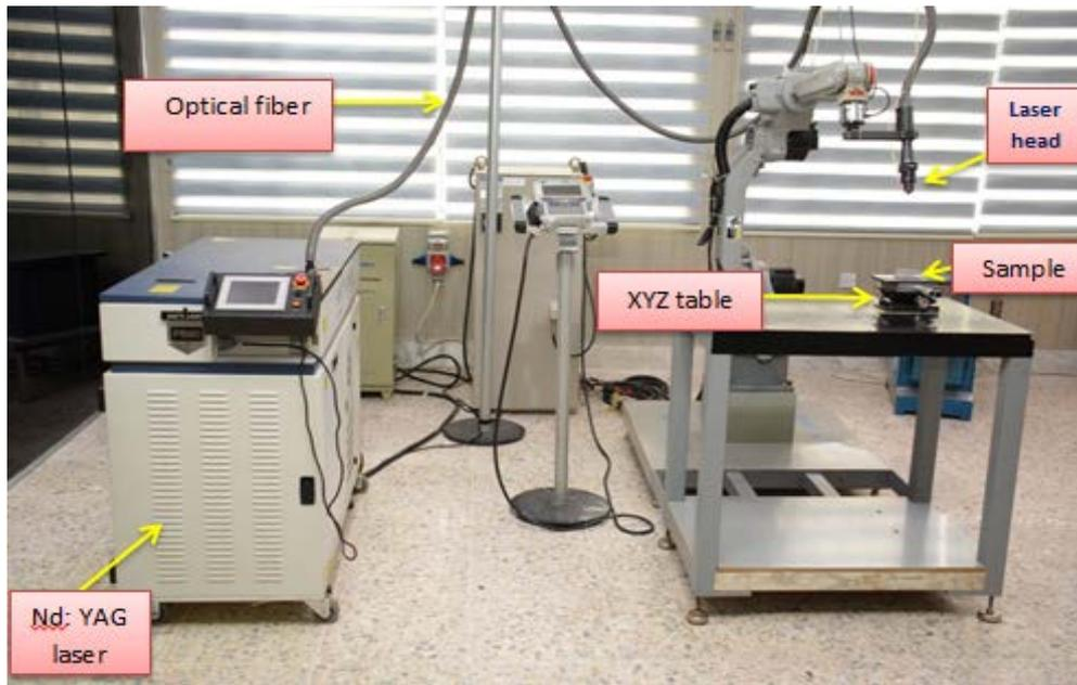
**Figure 2: the experimental setup of preplaced laser cladding**
