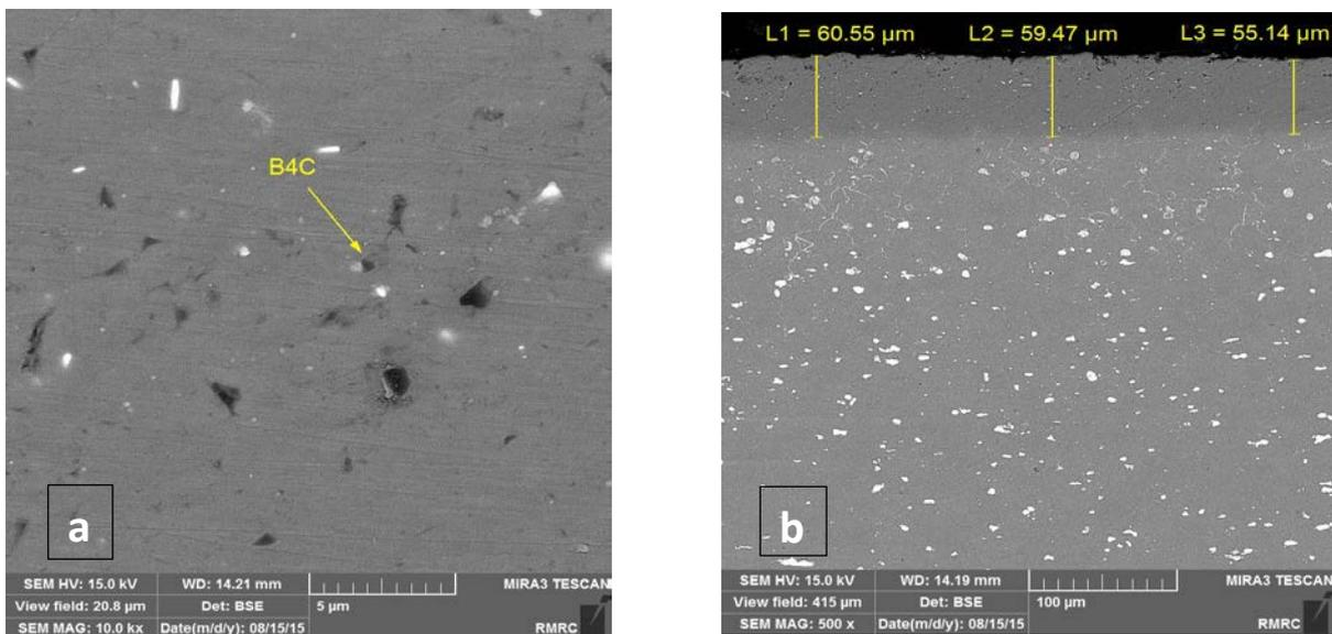
**Figure 3: (a) SEM of 2024 Al-alloy cladded with B<sub>4</sub>C powder; (b) SEM for the cross section of SEM of Al 2024 with B<sub>4</sub>C**
