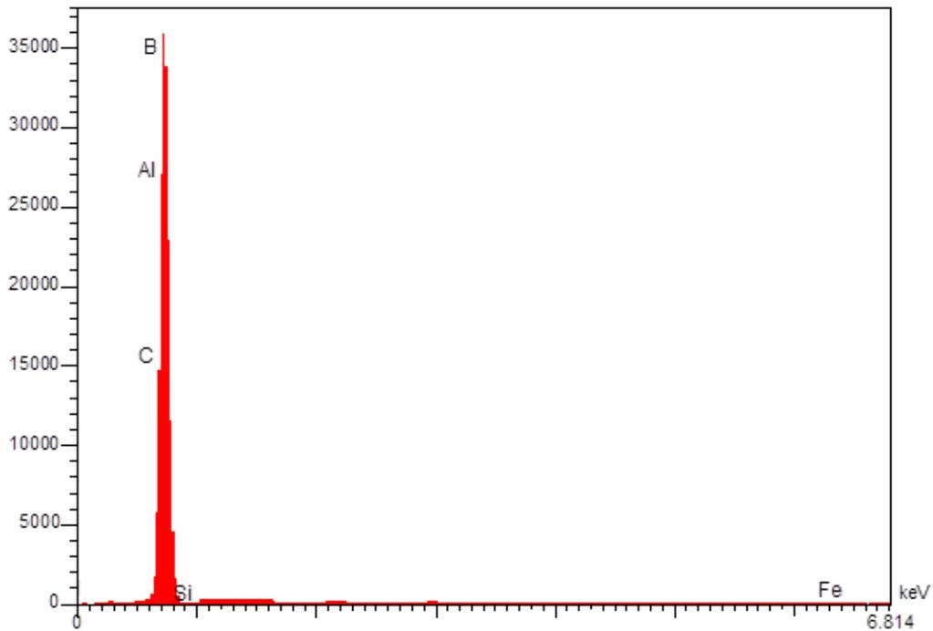
**Figure 6 : EDS for Al 2024 clad with B<sub>4</sub>C**
