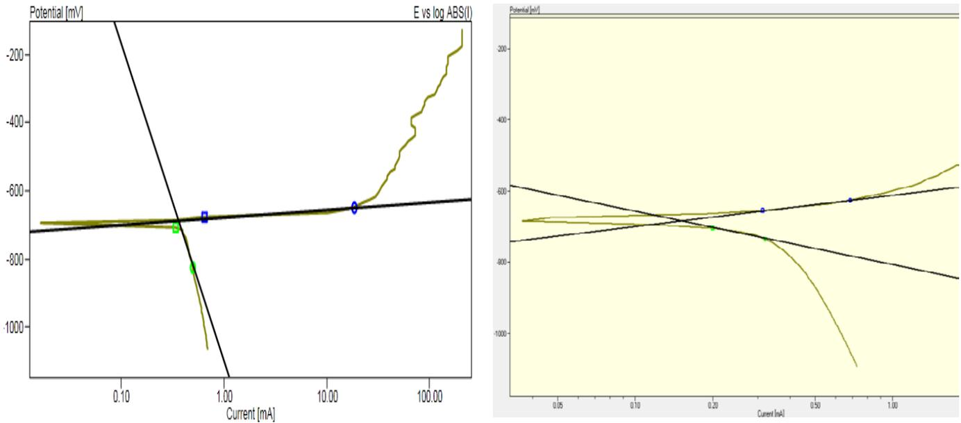
**Figure 5: (a) Corrosion test of pure Al 2024 alloy ( $I_{corr} = 362\mu A$ ); (b) Corrosion test of Al 2024 alloy with B<sub>4</sub>C ( $I_{corr} = 152\mu A$ )**
