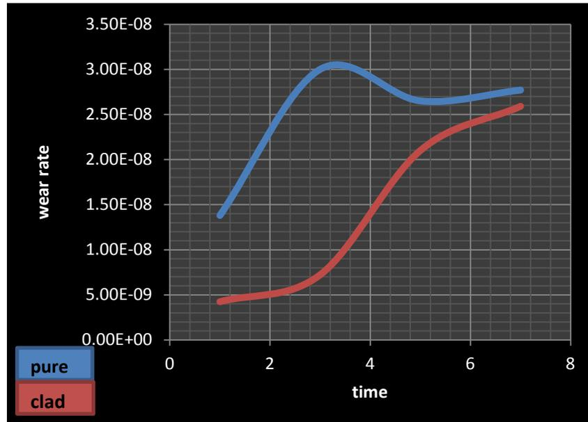
**Figure 7 Wear test Al (2024) alloy with B<sub>4</sub>C cladding**
