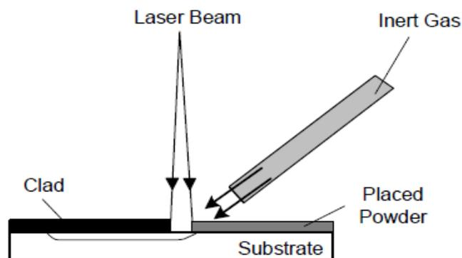
**Figure 1 : the schematic of preplaced laser cladding**
