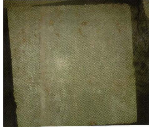
Fig.No 4 Precipitation on Surface of Concrete Cube.
