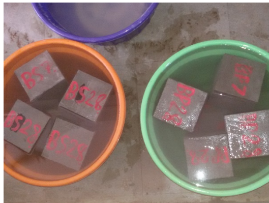
Fig No. 2 immersion of Sample in Precipitation of Media
