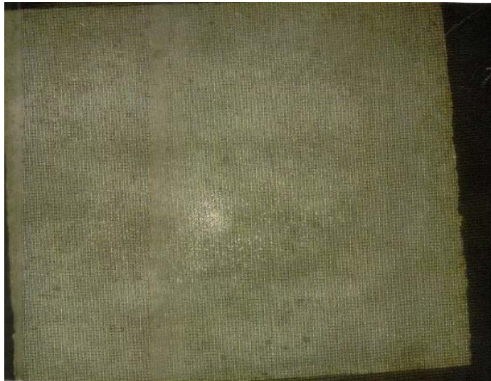
Fig no. 5 Precipitation on Surface of Concrete Cube.
