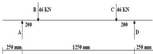
Fig 2.1: Load distribution Diagram for Tractor trolley
