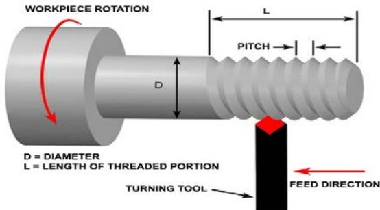
Fig -03: Turning operation
