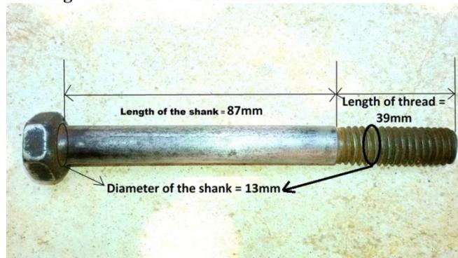
Fig -02: Dimensions of the bolt
