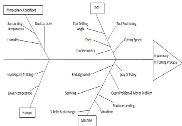
**Fig -5:** Cause and effect analysis (Fish bone diagram)
