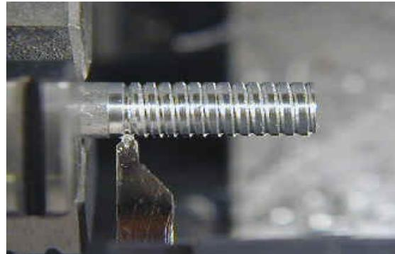
Fig -04: Threading operation on lathe machine
