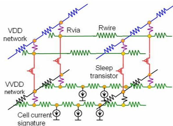
Fig.2: Sleep transistor power network
