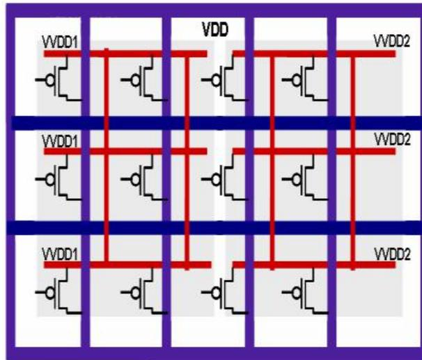
Fig.1: Distributed sleep transistor implementations
