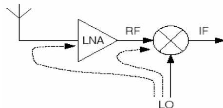
Fig.2 LO to RF leakage
