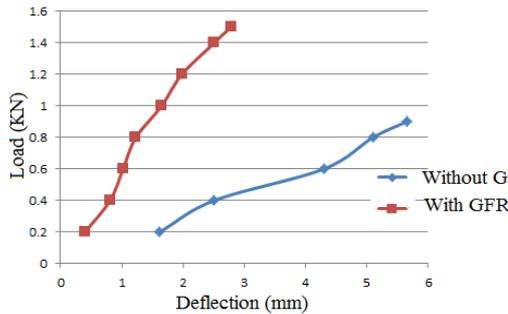
Graph 3: Load vs. Deflection for without and with GFRP specimen (7days)
