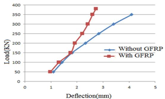
Graph 2: Load vs. Deflection for without and with GFRP specimen (28days)
