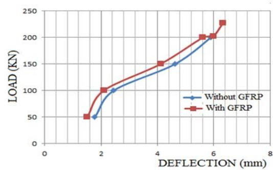
Graph 1: Load vs. Deflection for without and with GFRP specimen (7days)
