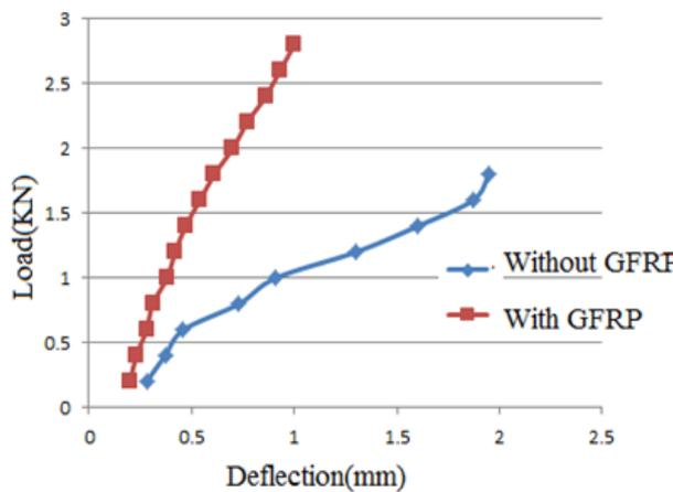
Graph 4: Load vs. Deflection for without and with GFRP specimen (28days)
