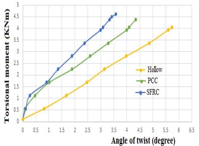
Chart -3: Torque twist response of Hollow, PCC & SFRC (7 Days specimen)
