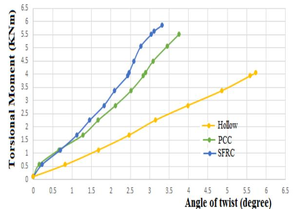
Chart -4: Torque twist response of Hollow, PCC & SFRC (28 Days specimen)
