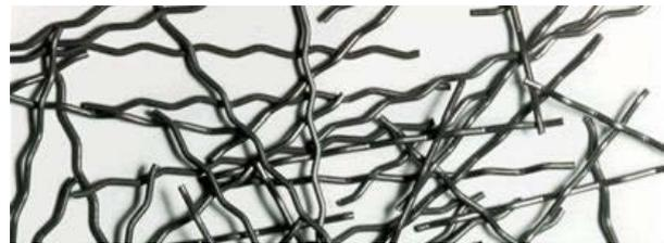
Fig 1: Steel Fibers
