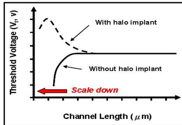
Figure 1 - Effect of Halo Implantation to  $V_{TH}$  values in CMOS Downscaling [5]
