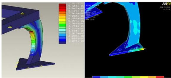
three-point linkage. The plate thickness for top link is kept as 10 mm and two plates are spaced at 50 mm spacing attached to each other with a spacer in between them. This arrangement was decided by considering hitching system of different 18 HP tractors.
