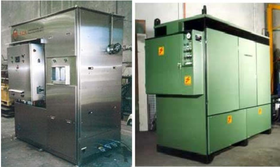
**120kW Electric Steam Generator & Superheater 300°C**
