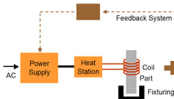
**Fig 1:** Typical Induction heating setup
