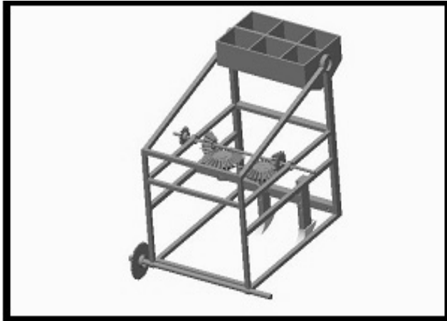
Figure 3: FRONT VIEW- Design of Seed sowing cum Fertilizer machine
