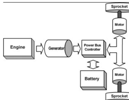
The driving system of the vehicle is responsible for most of the braking process. As soon as the driver steps onto the brake pedal of the vehicle (either hybrid or electrical), the brakes put the vehicle's motor in the reverse mode enabling it to run backwards causing the wheels to slow down. While in the reverse mode, the motor operates as an electric generator feeding this electricity into the vehicle's batteries.
