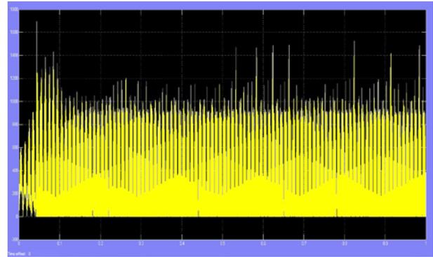
Fig 4 Terminal Voltage across MOSFET
