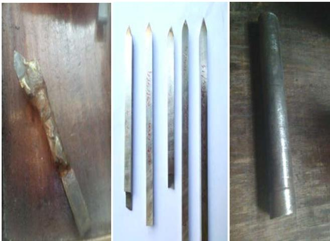
Fig. 3: Cutting tools and workpiece used during turning test [16]
