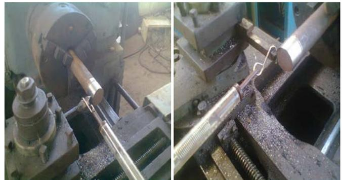
Fig. 4: Dry orthogonal turning process of mild steel sample and cutting force measurement using dynamometer [16]
