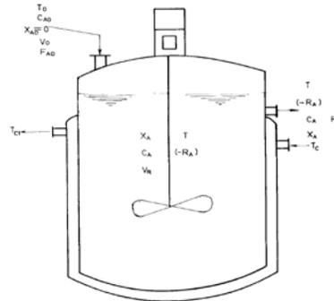
**Fig. 3 Hypothetical model of a Jacketed CSAT**
