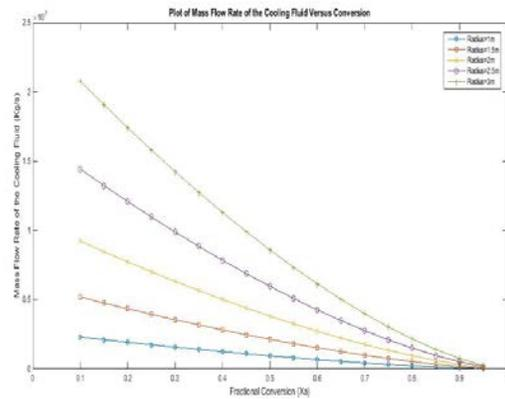
**Fig 7: Mass Flow Rate of Cooling Fluid versus Fractional conversion.**
