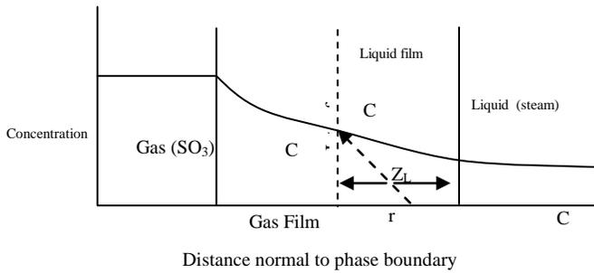
**Fig 2: Absorption with chemical Reaction**
