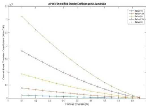
**Fig 6. Overall heat transfer coefficient vs conversion**
