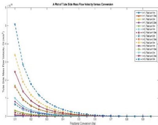
**Fig. 9: Tube Side Mass flow Velocity versus fractional conversion**
