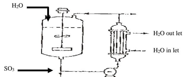
**Fig 4: Hypothetical heat exchanger rating unit.**
