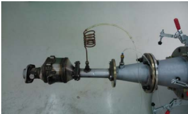
Fig. 1 Converter - Back pressure measurement test setup
