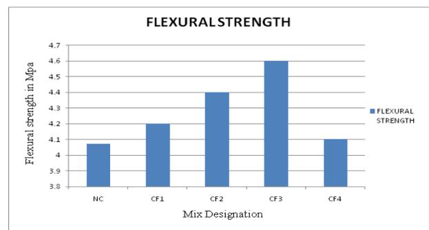
Figure 5: Variation In Flexural Strength
