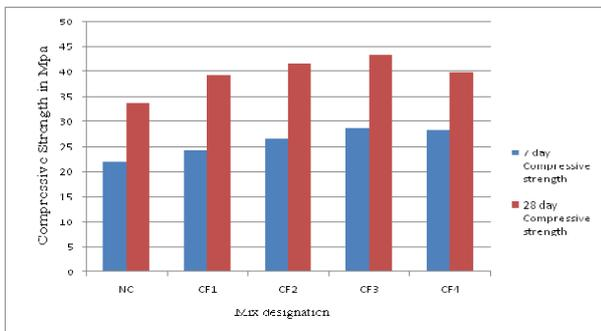
Figure 3: Comparison Of 7 & 28 Day Compressive Strength
